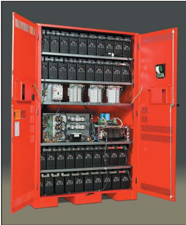
**The Illuminator Series IE** is an interruptible lighting inverter. It transfers to inverter mode (battery power) when utility power is interrupted for more than one line cycle. This series is capable of supporting full capacity of normally off load. The series E is best suited for fluorescent and incandescent lighting loads and systems that require large lighting loads that are normally off (illuminate during emergency conditions).
